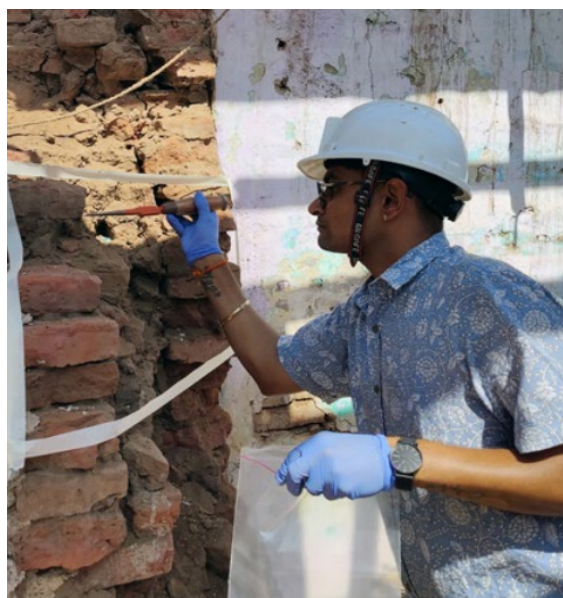
NDT tests at Kalidas Jethabhai House (photograph by Audrey Alvares), Sample collection (DRP report)
